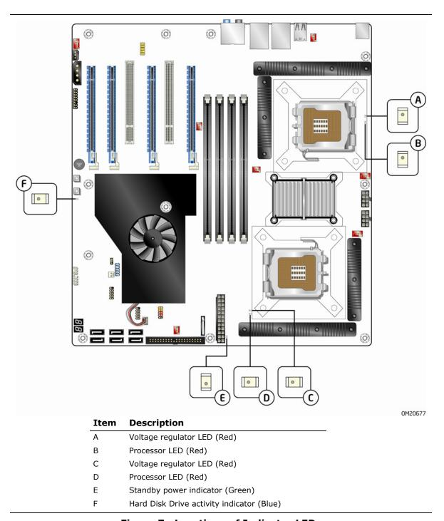
**Figure 7. Locations of Indicator LEDs**
